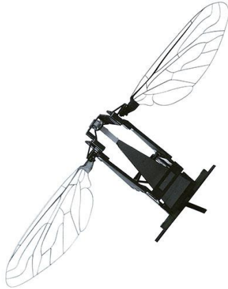
Figure 3. Pico aerial vehicle (RoboBee (Wood et al., 2013))
